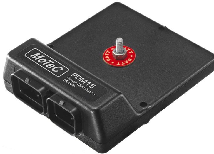
MoTeC's 15 output Power Distribution Module is designed to provide electronically switched power to various electrical systems in the vehicle such as motors, lights, solenoids, and electronic devices such as ECUs and data acquisition systems.
