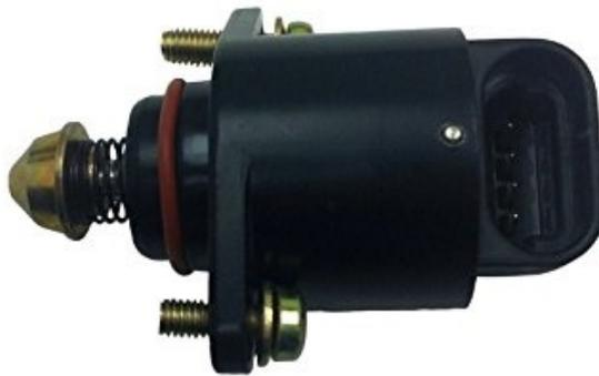
There are two general types of stepper motors that can be identified by the number of pins: firstly the General Motors style with four pins and secondly the Japanese style with 6 pins. Both stepper motors essentially work the same way. The six wire has additional power supply wires but the same number of control wires.
