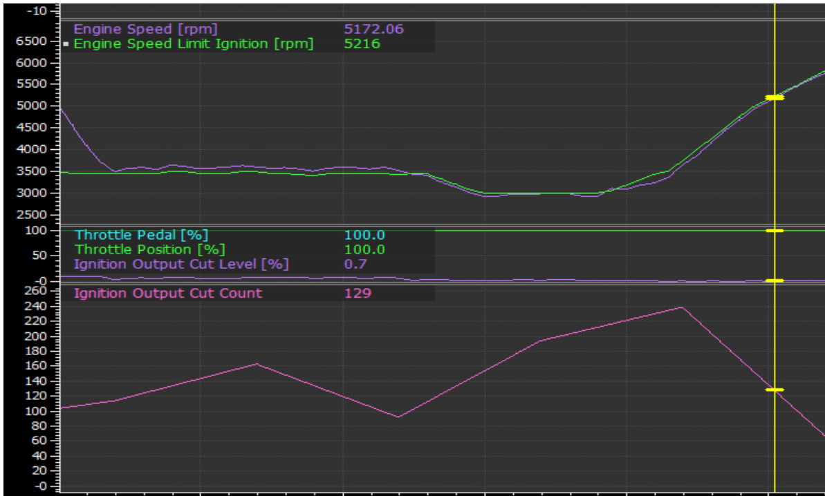
Data logging capture showing the Engine Speed being limited by the Engine Speed Limit Ignition during a launch. As can be seen in the magenta trace, the Ignition Output Cut Count is also increasing at the same time.
