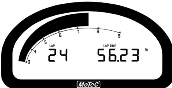
The Race display is normally used to display minimal information, e.g. RPM, Lap Time, Fuel Remaining or Laps Remaining.
